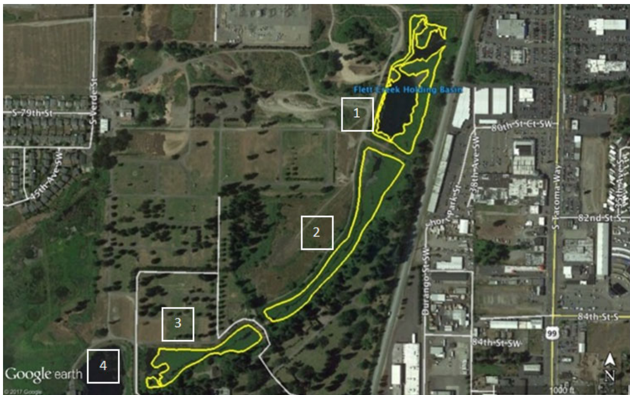
Figure 1. Flett Creek stormwater retention ponds with emergent/surface aquatic vegetation outlined.
