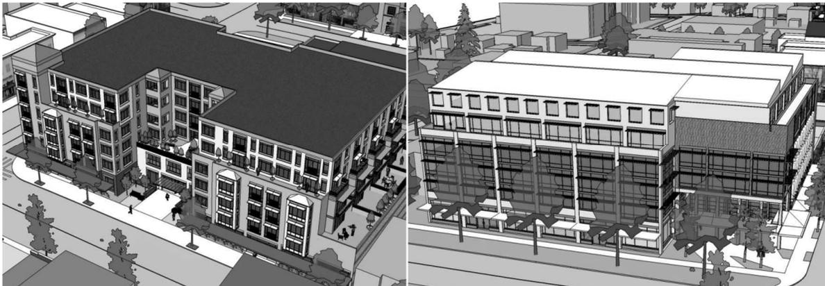
*Examples of façades wider than 120 feet that effectively use techniques to reduce the apparent bulk and scale of the structure. The image on the left uses street and upper level courtyards whereas the right image uses both vertical building modulation and the use of contrasting building materials and articulation.*
