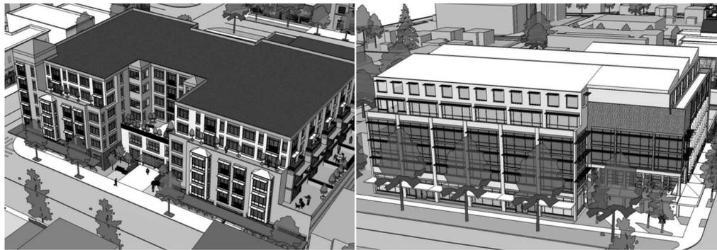
*Examples of façades that effectively use techniques to reduce the apparent bulk and scale of the structure. The image on the left uses street and upper level courtyards whereas the right image uses both vertical building modulation and the use of contrasting building materials and articulation.*
