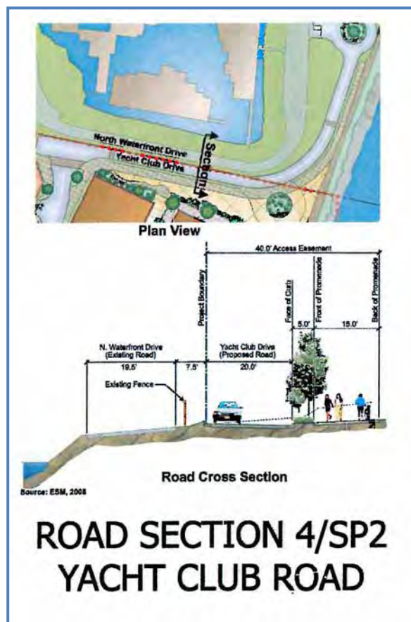
2.4 Missing Link: Conceptual cross-section of road improvements to accommodate a future promenade extension.
