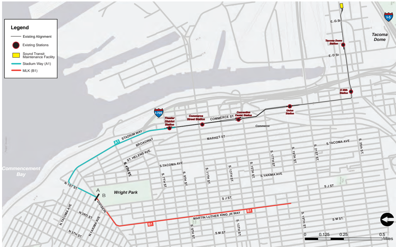
FIG. 8-15 SELECTED ALIGNMENT FOR THE TACOMA LINK EXPANSION
