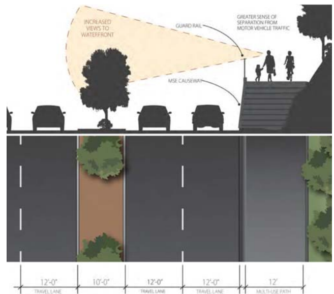
FIG. 8-18 A conceptual rendering from the 2013 Schuster Parkway Promenade Conceptual Design Report illustrating the recommended configuration for the Schuster Parkway Promenade, an elevated causeway.
