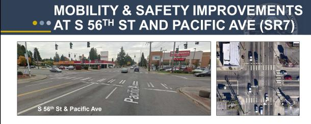
Project Detail: This project will upgrade all four corners of the intersection of S 56th and Pacific Ave with curb extensions, ADA-compliant curb ramps, and accessible pedestrian push buttons.
