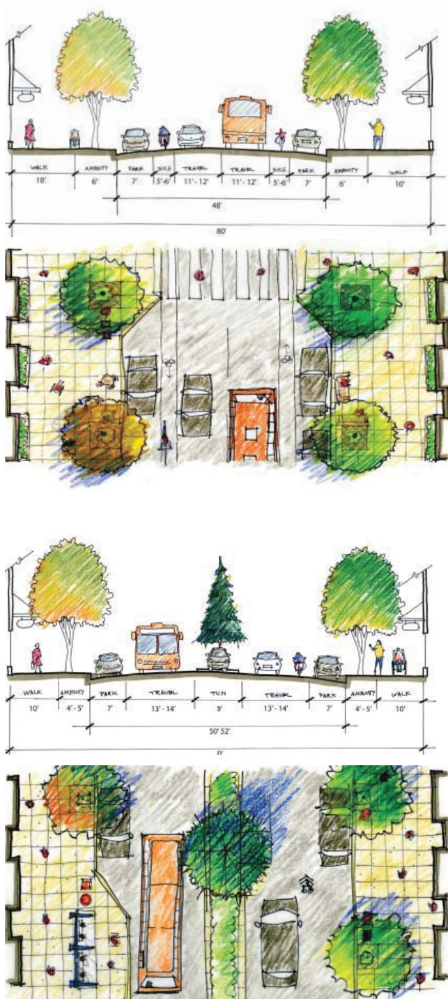
FIG. 9-19 Diagrams from Tacoma's Complete Streets Design Guidelines ; two-lane "Main Street" above, and transit priority street, below.
