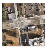
Project Detail: This project includes Fawcett Ave between 6<sup>th</sup> Ave and S 19<sup>th</sup> Street. It includes adding a bike boulevard and bike lanes, including curb ramps, pedestrian refuge islands, upgraded crossing equipment, bicycle detection, Accessible Pedestrian Signals (APS), mid-block crossings, traffic calming, and bicycle amenities.
