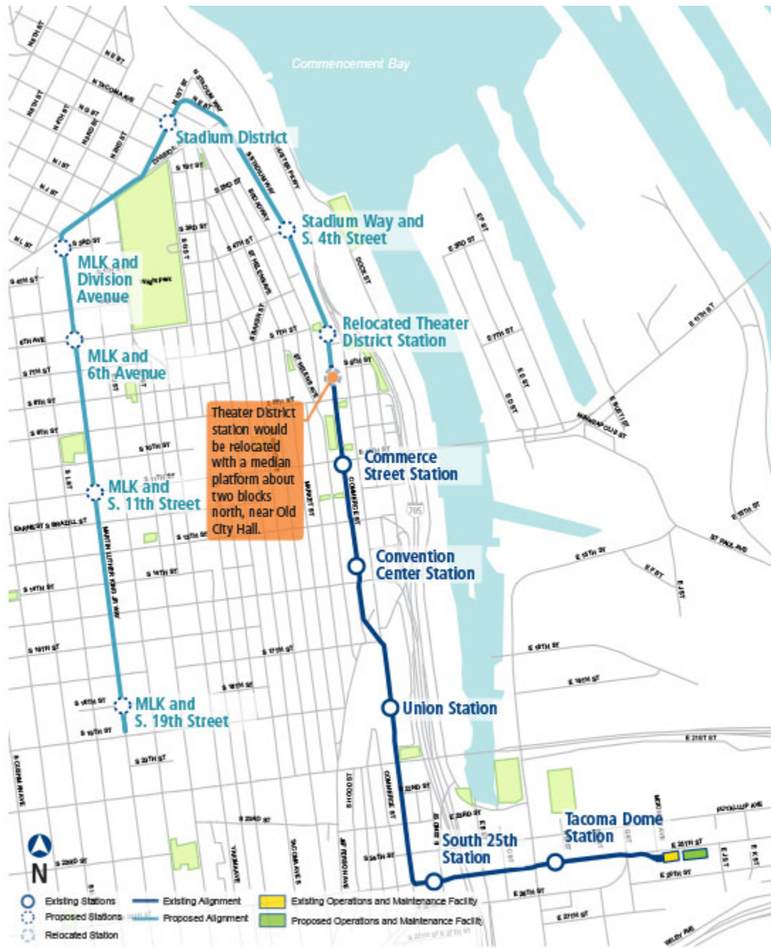
Figure 1 – Tacoma Link Expansion Alignment
