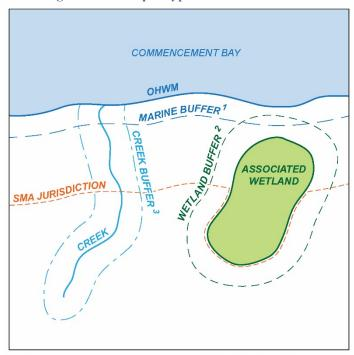
Figure 6-1. Multiple Types of Shoreline Buffers
